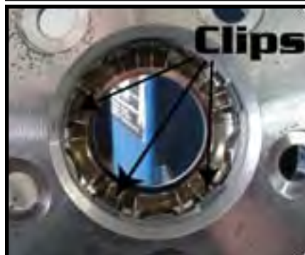
Clad wheel - inside - cone from this side with a standard taper cone and you hit the retaining clips, or hit the rear surface of the cladding
